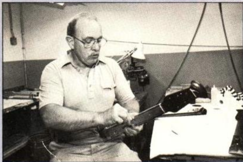
Above: Once the neck is complete the binding is sanded smooth. Right: The workman checks for high and low frets by using a straightedge (note that the beadstock is "weighted" to mimic the pull of the strings). Then a sanding block is run over the level frets to smooth any rough edges.
