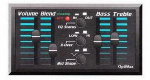
A microphone adds ambience and "breathy" highs — a nice "finish" to the on-board pickup sound. The OptiMax takes the concept to a new level with a special mike and blend control that give you the best of both worlds.
