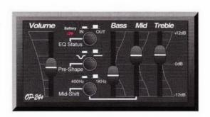
The famed Ovation OP-24 has been updated using the latest in low noise analog circuitry plus a "three-and-a-half" band equalizer. It also features a Pre-Shape circuit that lifts the bass and treble and reduces the "rumble" below 40Hz.
