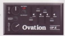
The OP-X features four precise bands of EQ (at 80Hz, 600Hz, 6.6KHz and 10KHz) to contour the sound accurately plus a very steep (30dB/octave) notch filter designed to kill feedback one note at a time. Now you can solve feedback problems without changing the character of the sound.
